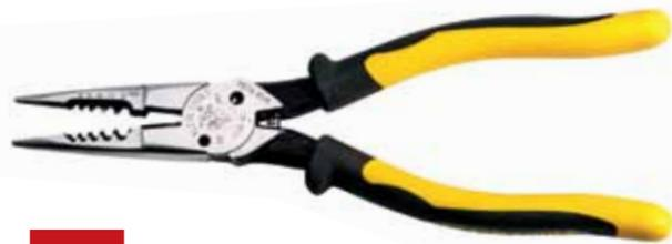
Klein's All-Purpose Pliers are built of forged steel with induction-hardened cutting knives for maximum durability. They can shear screws and strip, cut and loop 8-16 AWG solid and 10-18 AWG stranded wire.
