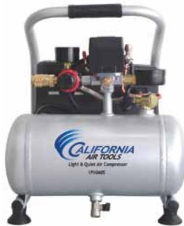
California Air Tools' Light & Quiet 1P1060S air compressor runs at just 56 decibels and delivers 1.20 cfm at 90 psi with a fast 15-second recovery time. Plus, it weighs just 29 pounds.
