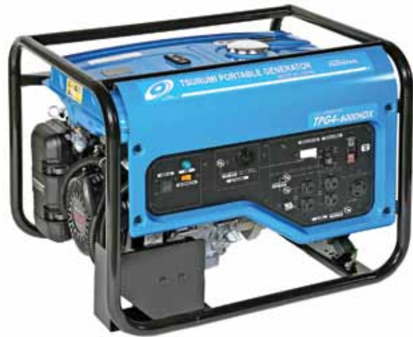
Tsurumi's model TPG4-6000HDX generator is powered by an 11-hp Honda OHV engine with a low-oil-level alert system, Automatic Idle Control and vibration reducing rubber pads on the engine. Its 6.6-gallon fuel tank delivers 8.2 hours of runtime.
