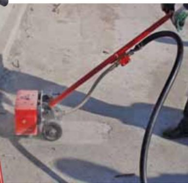
CS Unitec's Trelawny MHS11 multi-headed concrete floor scabblers produces seven times less vibration than standard models thanks to a three-point mechanical vibration damping system.
